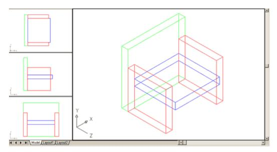
You don't need to dimension this drawing, but use the **Distance** command to confirm that the sizes are correct.
