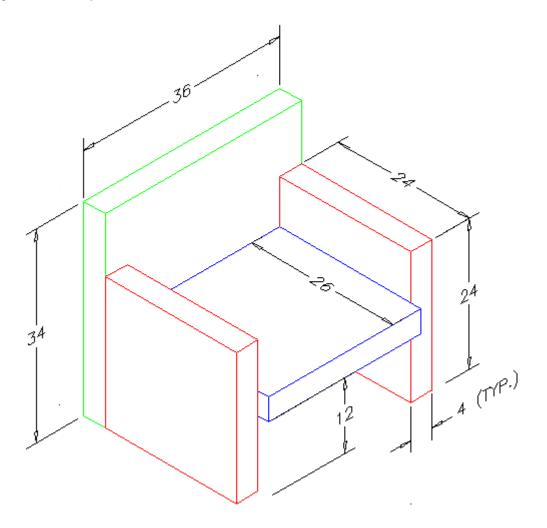
Start with the back. Make rectangle to define the plan view of the back of the chair. Copy it 34" in the Z-axis and then connect the corners with vertical lines.
