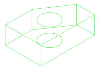
Pick any line and snap to an endpoint grip. Look at the coordinate display on the left of your status bar and see if it makes sense to you. Try this at other points. What you have just done is created a simple object in 3D drawing space. It has length, depth and height. Get used to looking at it, and review what you did to create it.
