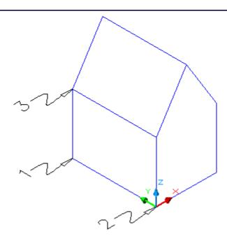
This is the '3-Point' option of the UCS Command. It is one of the most useful, because you control exactly where the new drawing plane will be. You must also be extremely careful when picking the 3 points, or your plane can be shifted and cause some major problems. I would recommend using this method for most of your UCS work - or at least get very comfortable with it before moving on to other methods.
